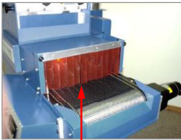
Tunnel Light Curtain
